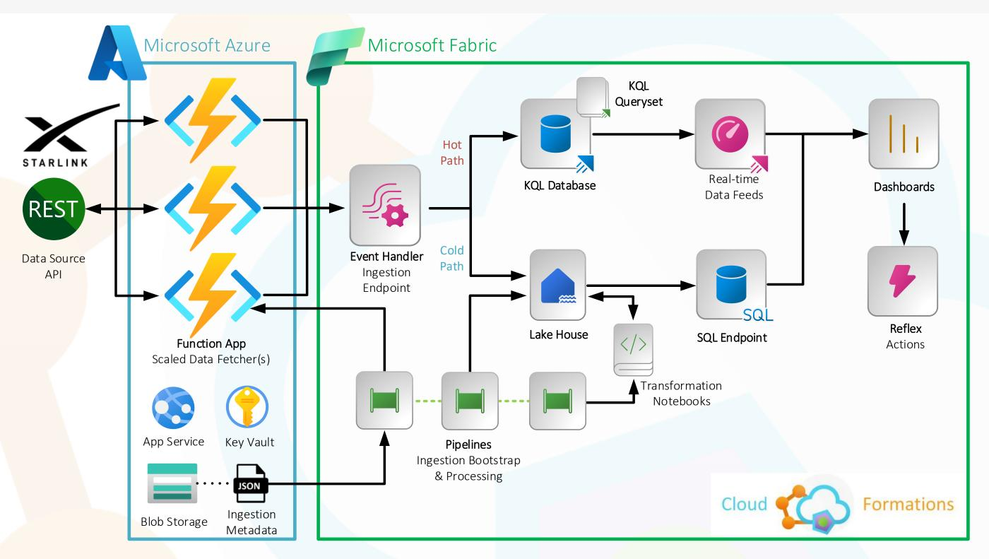
The greenfield implementation follows a microservices approach to data handling, leveraging Azure Functions Apps to ingest telemetry from the Starlink API at scale and metadata driven, feeding into a Microsoft Fabric Event Stream. Bootstrapped by Integration Pipelines, data feeds into Realtime Analytics Kusto Databases and Lakehouse structures for reporting using Power BI Dashboards.
